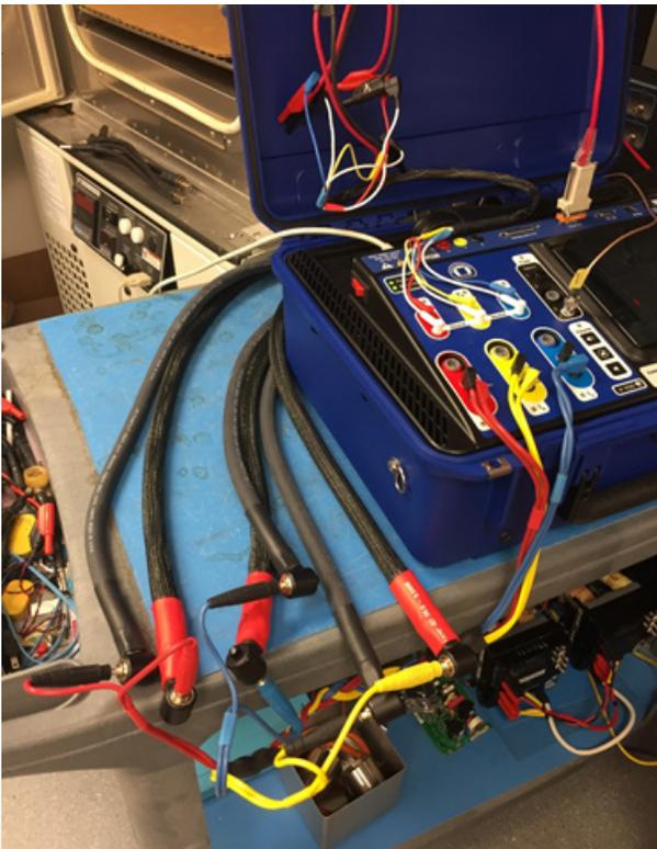
1. Connect the voltage cables to the 703/933 as shown, with the colored cables corresponding to each phase:
