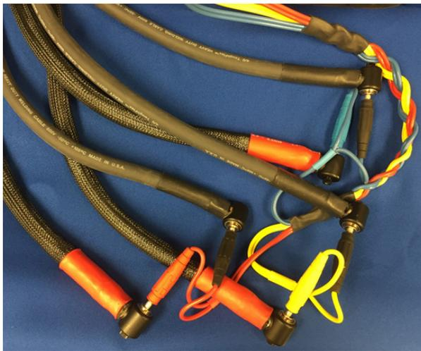
2. Connect the current cables to the 703/933 as shown, with the colored cables corresponding to each phase:
