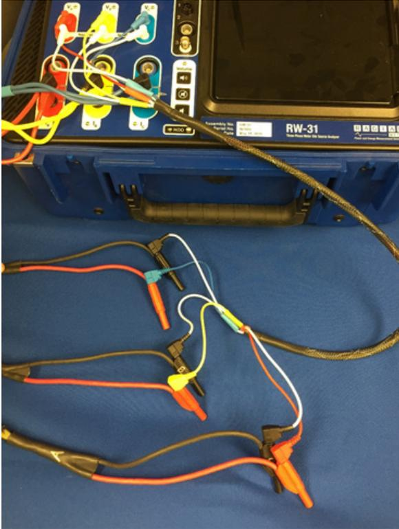
2. Connect the current cables to the 703/933 as shown, with the colored cables corresponding to each phase:
